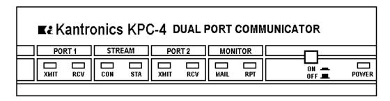
The front panel has a power switch and nine LEDs. There are eight LEDs used as operating status indicators and one for power. The front panel is divided into four sections, each section containing two operating status LEDs. Each section is separated by a white color bar. Each LED has the function indicated below:
