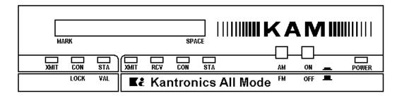
The front panel has two switches, eight LEDs and a ten segment LED bargraph. There are seven LEDs used as operating status indicators. The front panel is divided into two sections. The left three LEDs are the indicators associated with HF operation, and the four right LEDs are the indicators associated with VHF operation. The two segments are divided by a white color bar. Each LED has the functions indicated below:
